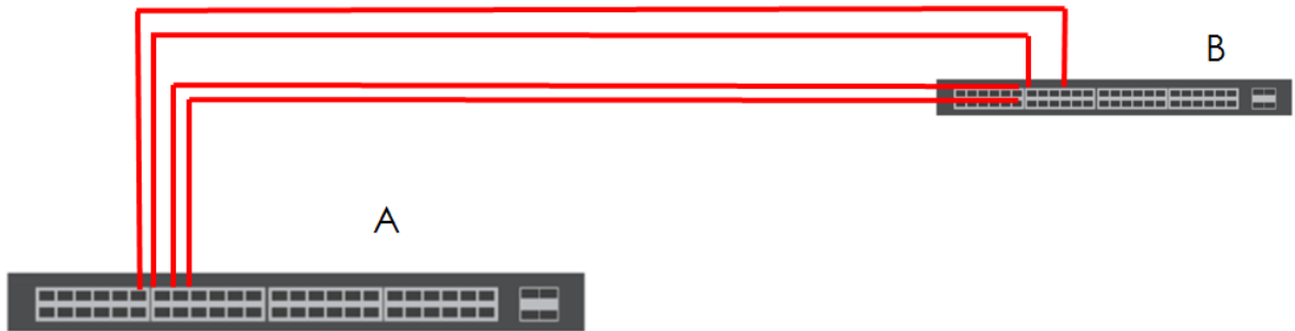
Figure 114 Trunking Example - Physical Connections
