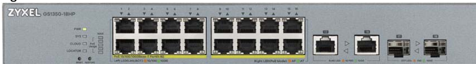
Figure 13 Front Panel: GS1350-26HP
