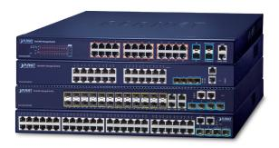
PLANET SGS-5240 series is a Layer 2+ Stackable Managed Gigabit Switch that provides high-density performance, **Layer 3 static routing** with **10Gbps uplink** interfaces delivered in a rugged, strong case.
