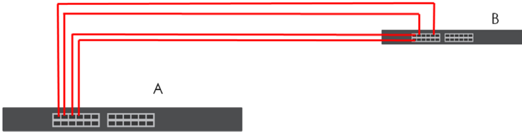
Figure 118 Trunking Example - Physical Connections
