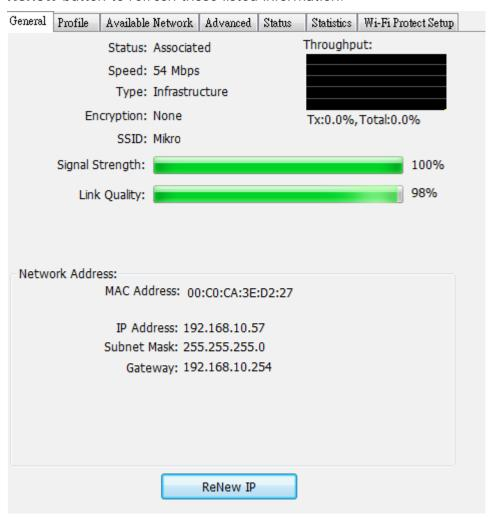
**Status:** Check if the device associated to target network.
