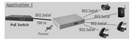
In Application -1, the PoE+ Extender Switch receives both power and data from uplink port that is connected to a PoE Switch. And four PoE PD devices are connected to PSE ports of the switch. In such application, one PoE connection is extended to four PoE connections and
