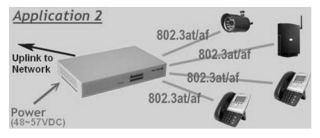
In Application -2, the switch cannot receive power from uplink port. A local power connection is provided for PoE application.
