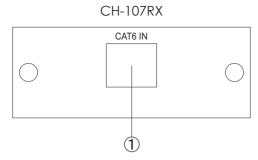
① CAT6 IN: Connect from the CAT6 output of the transmitter with a CAT6 cable to the CAT6 input of the receiver.
