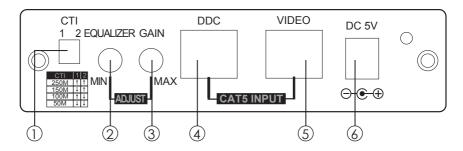
① CTI dip switch – To optimize the CTI use the twin switches to set the operating distance.
