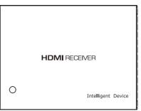
(1). Power LED: The blue LED will illuminate when the device is connected with power and detected the signal.
